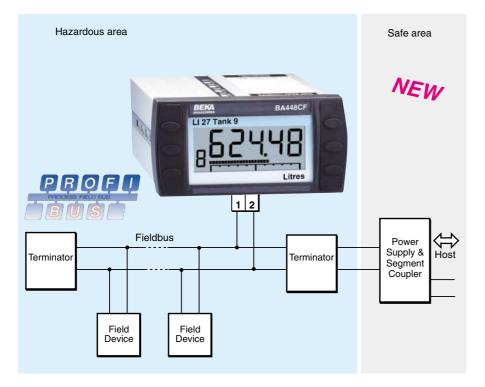
The BA448CF-P PROFIBUS Indicator is an intrinsically safe instrument that can display up to eight fieldbus process variables within a hazardous area. A numeric annunciator on the left hand side of the screen shows which variable is being displayed. This version of the indicator supports PROFIBUS PA protocol; for FOUNDATION<sup>™</sup> fieldbus systems an alternative version is available – please see BA448CF-F FOUNDATION<sup>™</sup> fieldbus datasheet.
